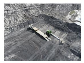
Mine operators must have controls in place to manage the risk of EWP's overturning during loading and unloading activities. EWP's should be matched appropriately to the size of the transport vehicle (length and width) and be centrally positioned on the deck or tray. Operators should plan loading and unloading tasks and final machine position before commencing the task.
