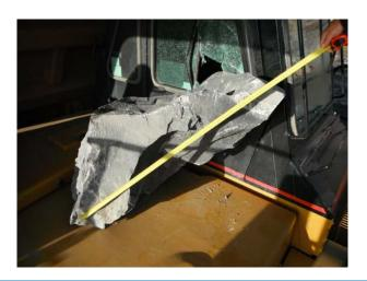
Dangerous incident SinNot-2018/01736 At an underground metalliferous mine, a worker was sitting in a parked light vehicle with the lights and beacon on. An underground loader entered the same level and when it turned right it clipped the light vehicle. No workers were injured and minimal damage was reported.
