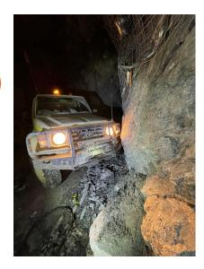
Vehicle operators must comply with correct park-up arrangements, particularly when parking on a grade. Mine operators should consider installing interlocks or warning systems for park brakes on light vehicles and other mobile equipment. Refer to Safety Bulletin: SB13-02 Unplanned movements of vehicles - too many near misses.
