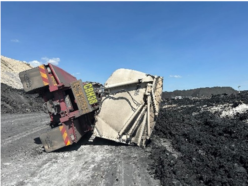
Picture 15. Rolled rear trailer.
