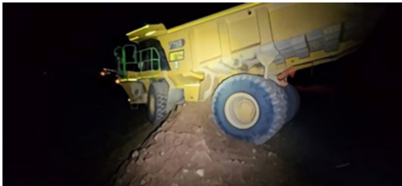
Picture 7. Haul truck on bund.
