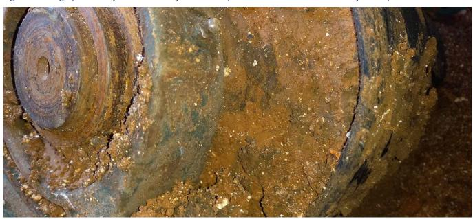
Guarding had been removed from the mobile screen by the workers for the purpose of cleaning mud off the tail drum of the mobile screen's main conveyor. The workers cleaned the tail drum by holding the edge of a standard garden spade against it as it rotated at idle speed. After scraping mud off the tail drum using this method, the belt speed was then increased to assist in tracking the conveyor belt to realign it.
