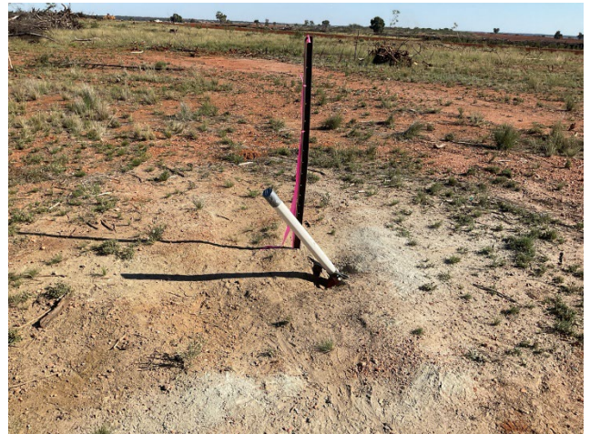
Figure 2 RC hole LTRC002 - partial rehabilitation, left open for further testing
