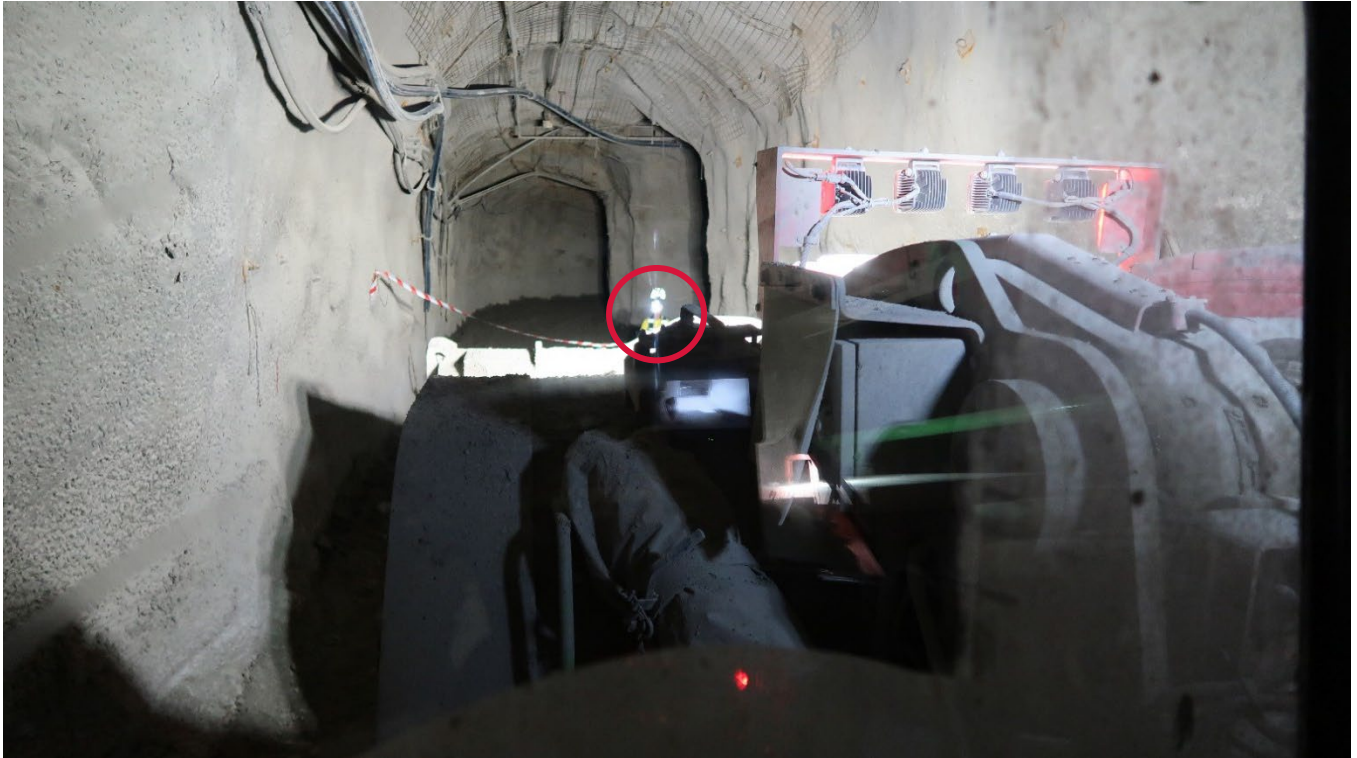
Figure 3: View from the operator's cabin of a worker (circled in red) standing 10 metres in front of the loader bucket during incident recreation. The worker was not visible to the operator at closer distances
