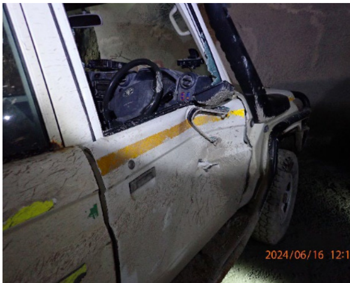
Picture 12: Light vehicle damage after incident.
