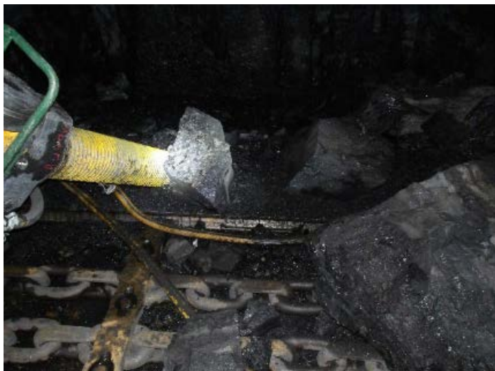
Picture 3. Spalled coal slab.
