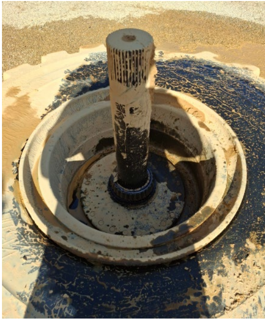
Figures 7 and 8: Loader drive shaft splines, and differential drive shaft retaining bolt and shims
