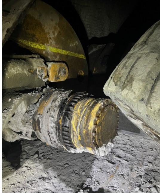
Figure 4 and 5: Loader wheel against wall, and intact wheel studs on hub
