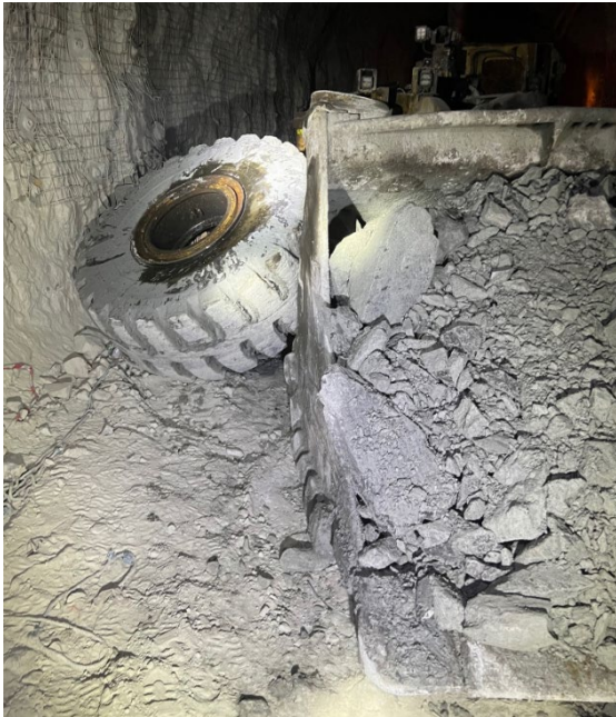
Figure 4 and 5: Loader wheel against wall, and intact wheel studs on hub
