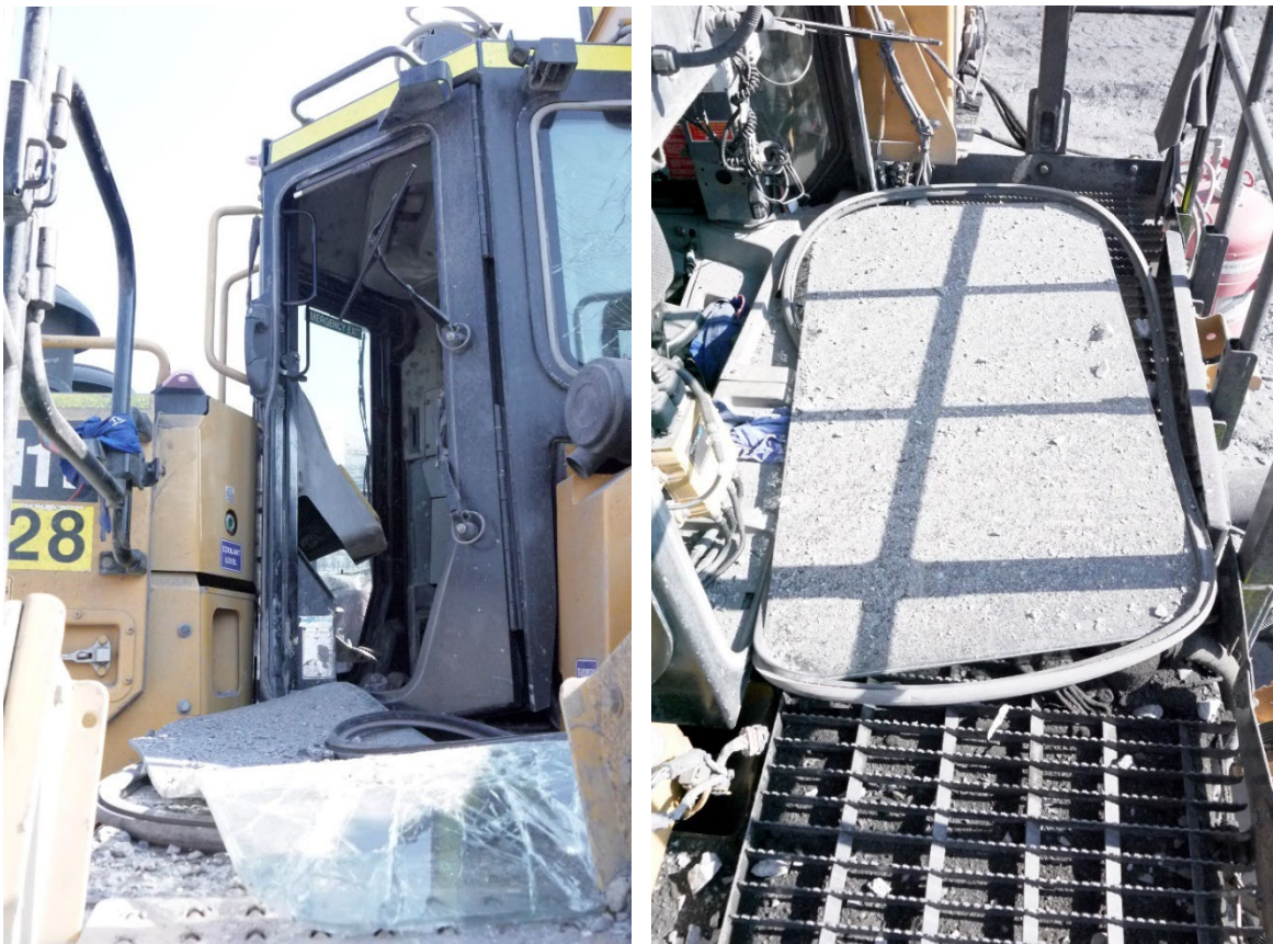
Figure 3: Damage to the dozer door (left) and rear window (right)
