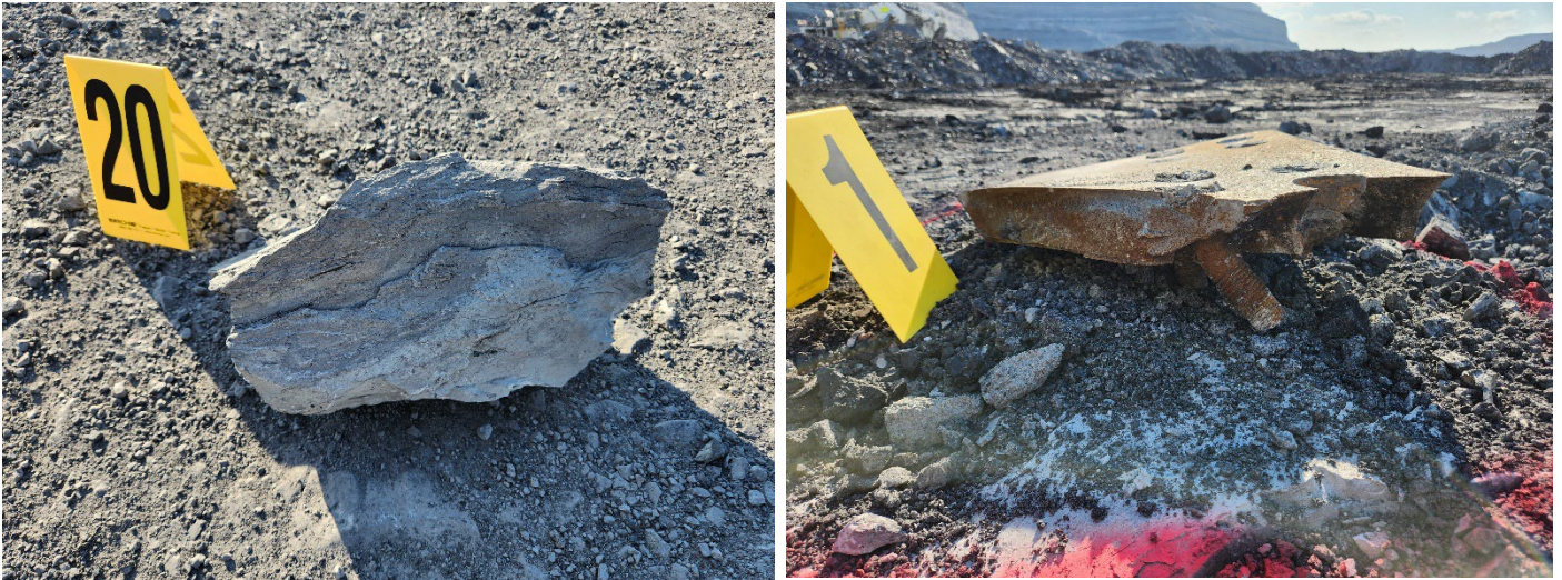
Figure 2: Some of the fly rock (left) and part of the dozer blade (right)
