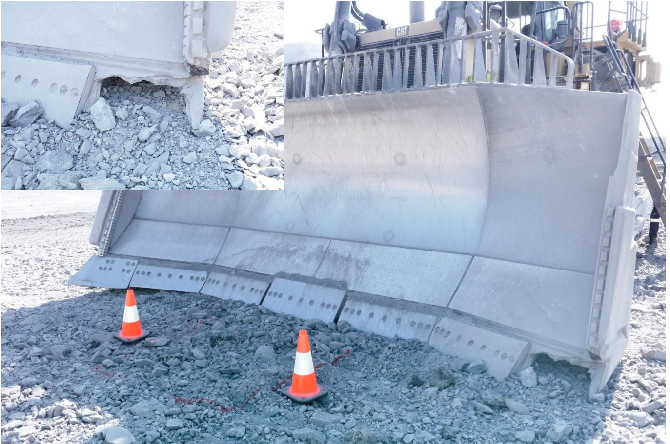
Figure 4: The blade of the dozer, showing damage to one side
