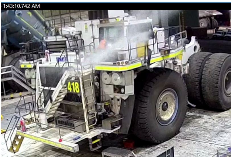
Figure 3: Release of uncontrolled energy - brake system hose whipping about releasing oil
