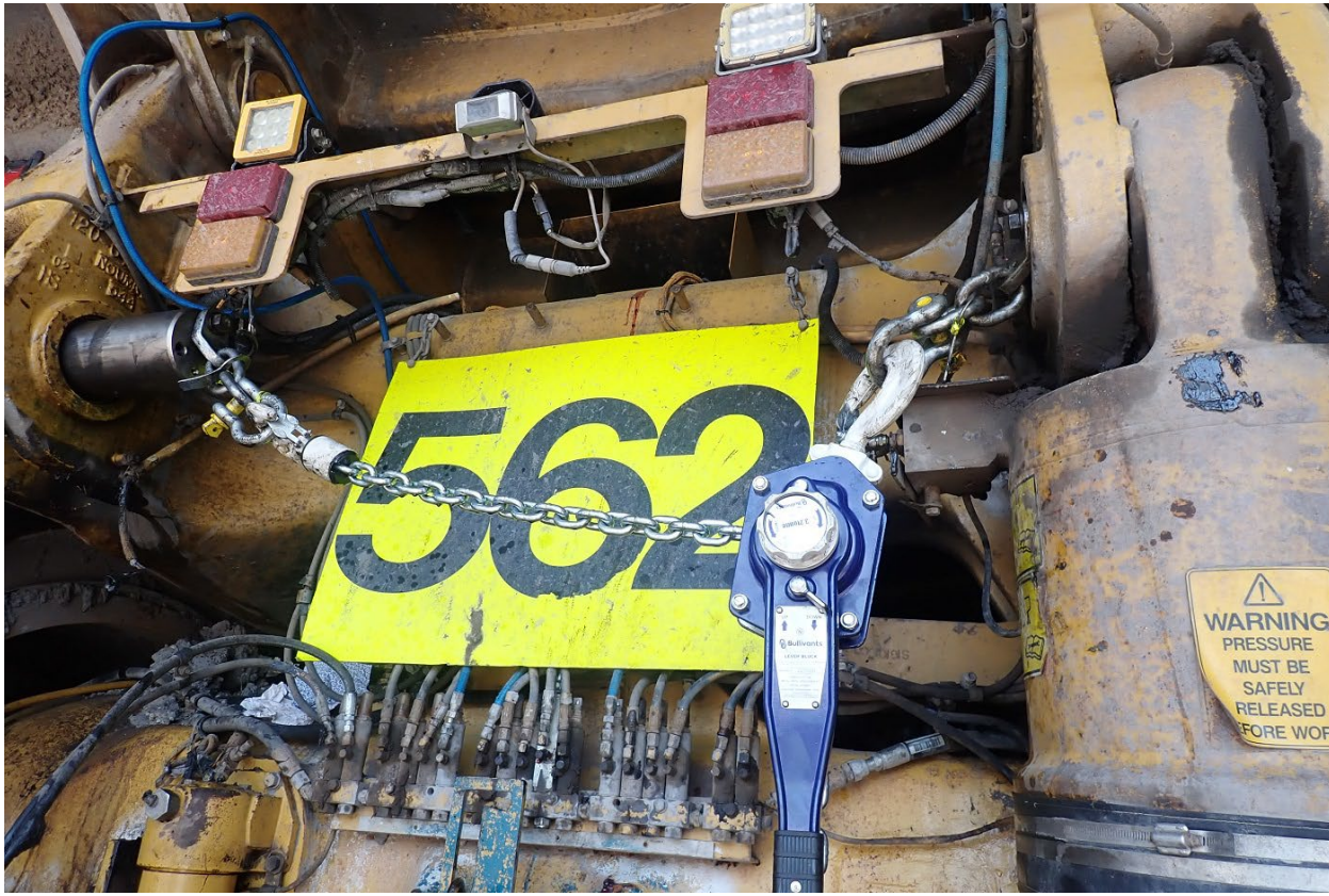
Figure 3: Lever block used to draw back the top pin
