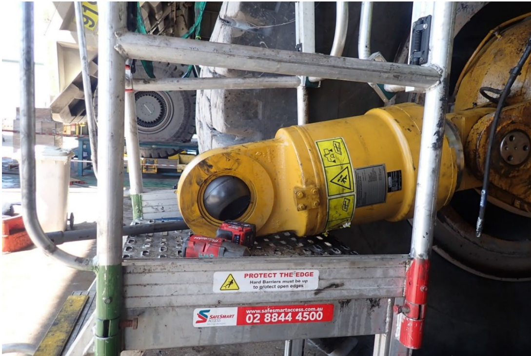
Figure 2: The strut where it came to rest after hitting the worker
