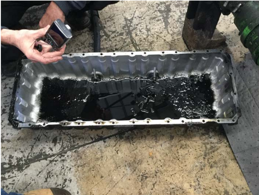
Figure 6: Debris found in sump (fragments of the piston skirt and conrod bolts).
