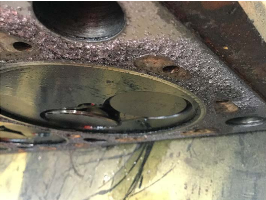
Figure 4: Valve head from No 6 is not seated indicating bent valve shaft.
