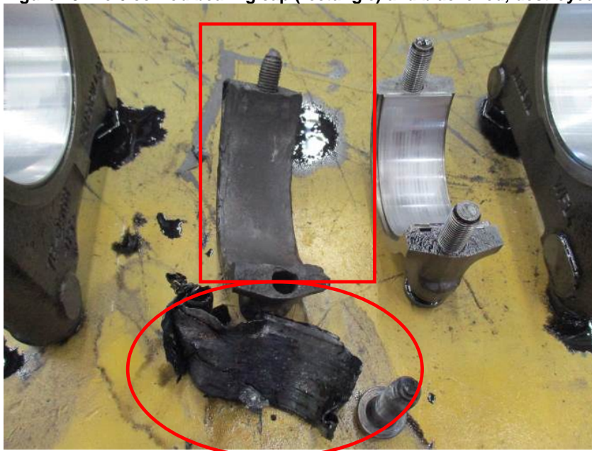
Figure 10: No 6 conrod bearing cap (rectangle) and blackened, destroyed No 6 bearing shell (oval).
