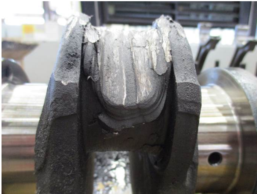
Figure 11: No 6 rod journal became so hot that impact with the connecting rod caused material flow and left an imprint of rod profile on the crankshaft.
