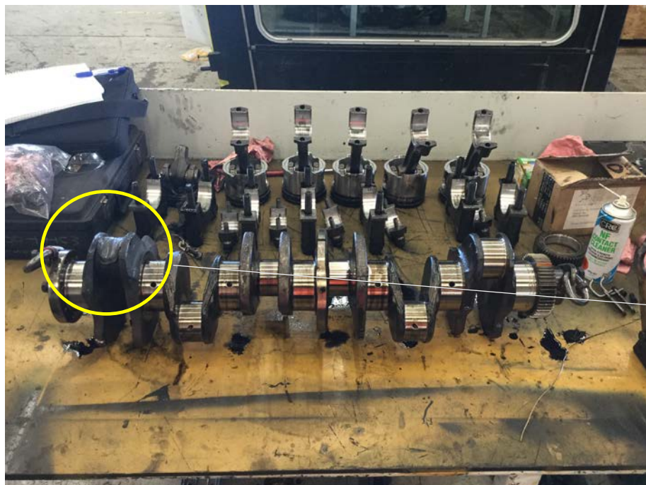
Figure 7: Crankshaft, main bearings caps and pistons complete with conrods (1-5) on bench. Can see No 6 blackened bearing journal.
