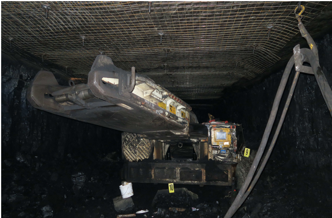
Figure 9 Continuous miner 806A panel ‘G’ heading as found by investigators
