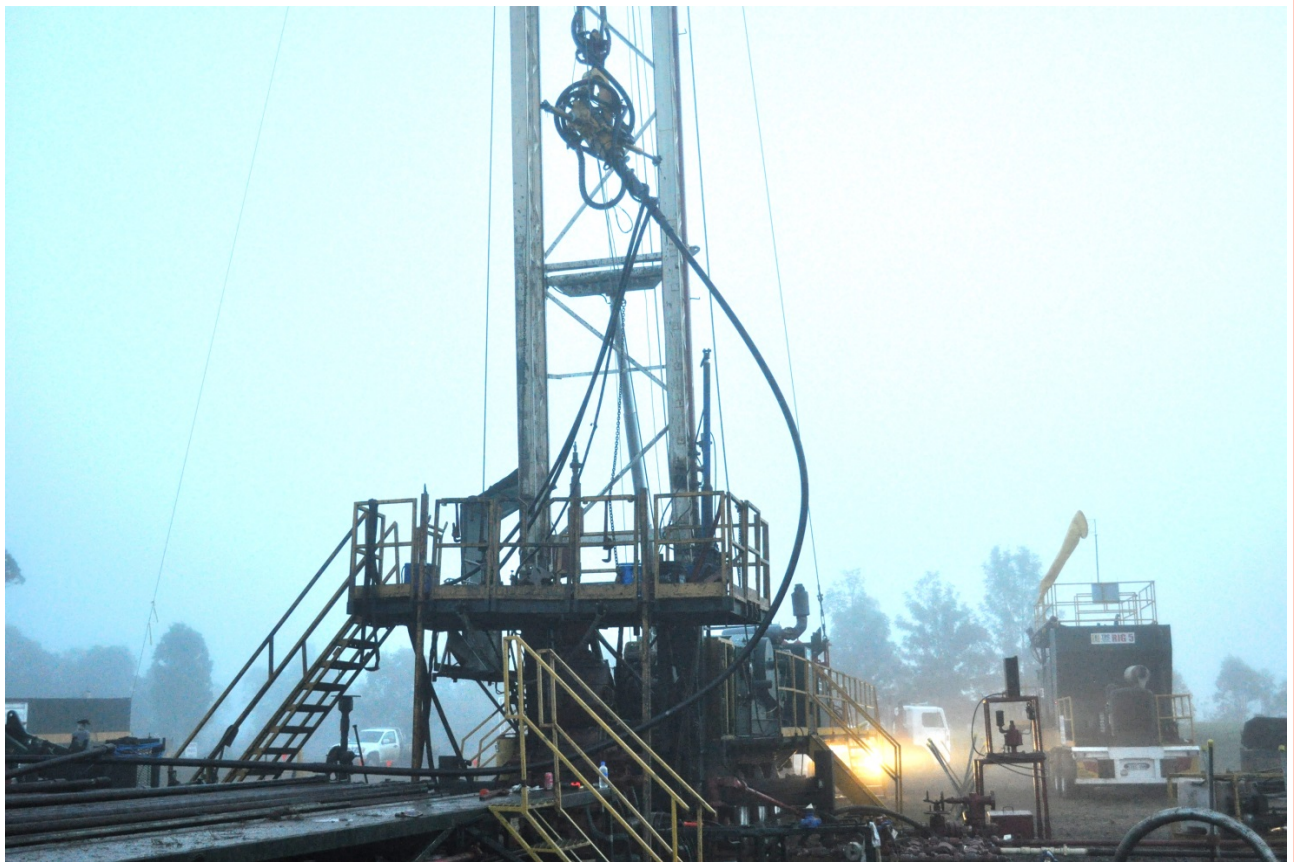
The workover rig showing the swivel and a portion of the ejected pipe Photograph supplied by Metgasco
