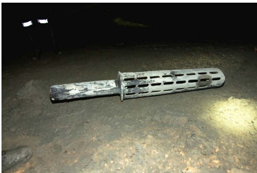
Strainer found in the vicinity - Photograph by Investigation Unit
