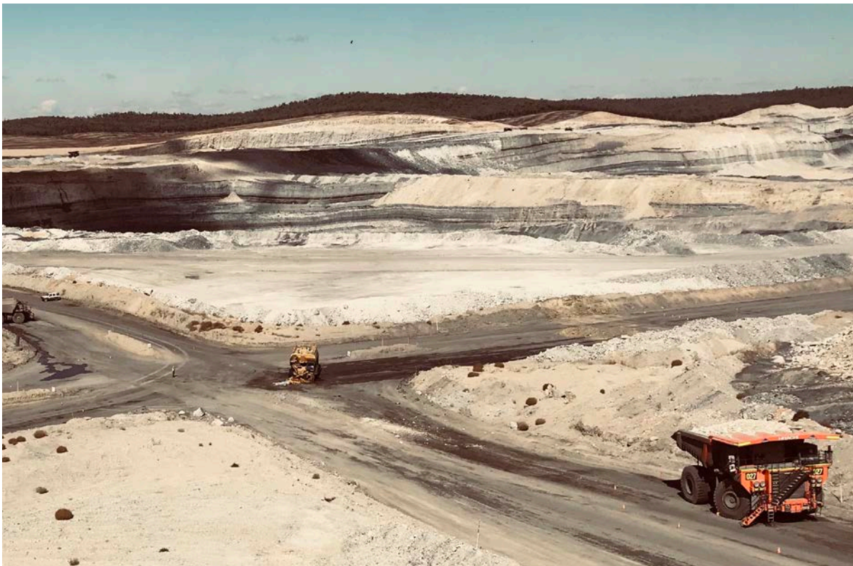
Photograph 2: Four-way haul road intersection showing trucks involved in the collision.
