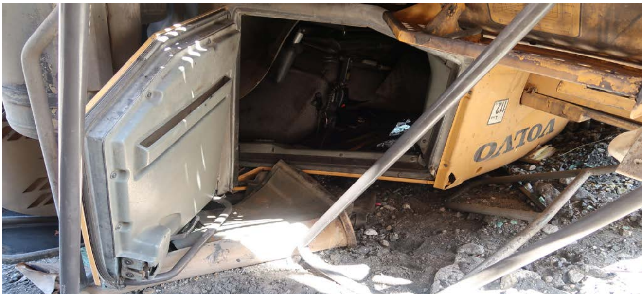
Photograph 2: The damaged cabin of the articulated water cart.
