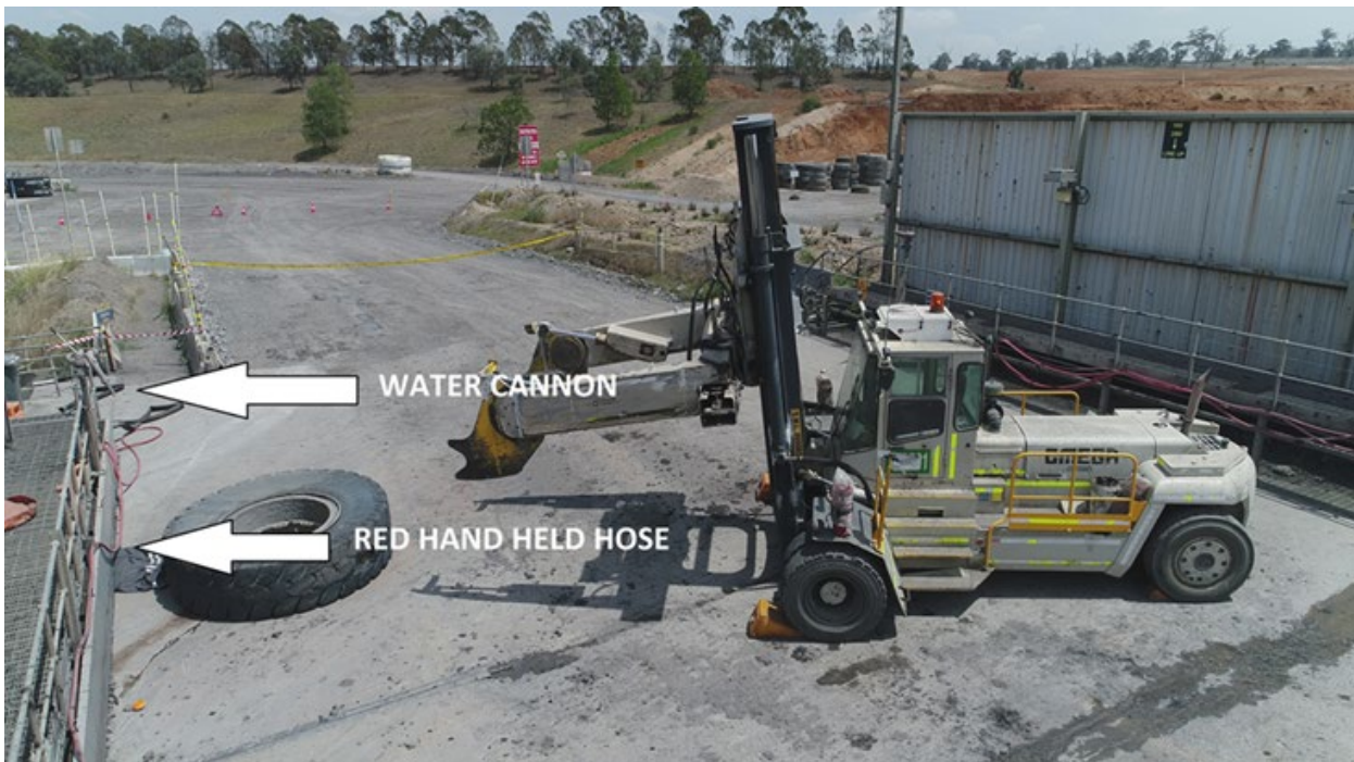
Figure 9 Heavy vehicle wash bay platform with water cannon and red handheld hose
