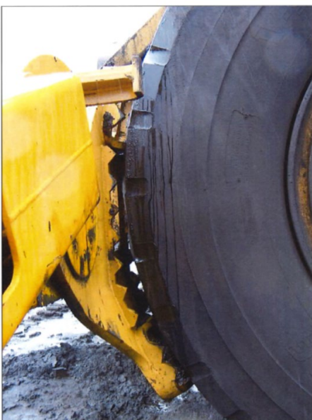
Figure 23 Profile of grabs on large truck tyre in vertical position
