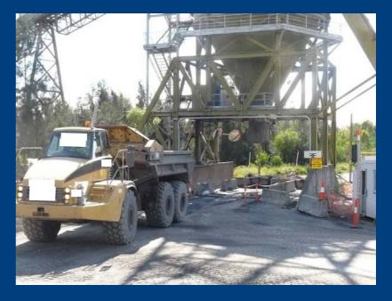
Post incident loading by reversing of FOPS cabin truck under chute
