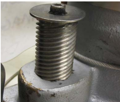
Photo 3. Jacking screw in a threaded case - ACCEPTABLE ARRANGEMENT
