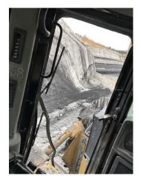
An assessment of the integrity of the highwall must be conducted prior to commencing work beneath the highwall. Consideration should be given to:
