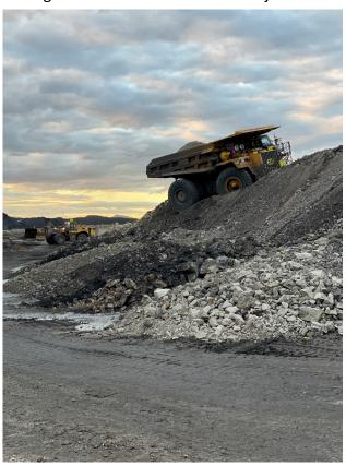
Mines should have systems in place to ensure windrow standards are regularly verified and maintained. Ground stability should be considered when planning a dump site.
