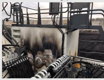
Inspections conducted after maintenance, particularly when hot work has been undertaken, should identify new hazards that may have been inadvertently introduced as a result of that task.
