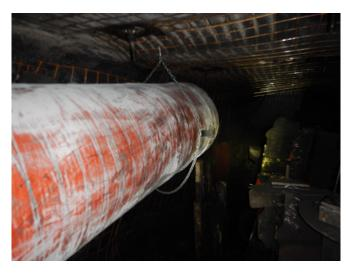
guards on the most inbye tube, to minimise the risk of workers being sucked into or against the ducting while working adjacent to it (e.g. on continuous miner platforms).
