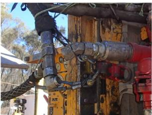
Daily inspections should include compressed air hoses, fittings and whip checks. Compressed air systems should be assessed for the risk of whipping hoses and controls, such as whip checks, should be put in place.
