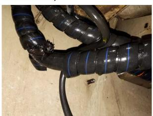
When conducting audits and assessing fuel sources, ensure hydraulic hoses outside the engine bay, as well as other ignition sources, are assessed and maintained to the same standards as those within the engine bay.
