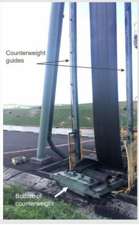
Operators of gantry conveyor systems should review the adequacy of restricted access areas under conveyors and near gravity loop take-up guides.
