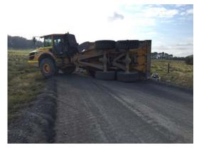
Operators of articulated dump trucks are reminded to drive to conditions and consider their experience level, prevailing light, tightness of corners, and gradients.
