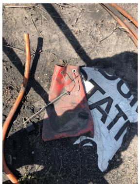
Dangerous incident IncNot0036558 Underground metalliferous mine During mining operations, a haul truck operator saw smoke, and then flames. He parked the truck and activated the fire suppression system. With the help of another two workers, they extinguished the fire with hand-held extinguishers. The fire was in the engine bay and articulation point of the truck.
