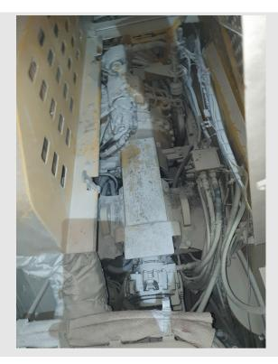
Dangerous incident IncNot0036556 Underground coal mine A worker suffered an electric shock while holding the hand rail of a continuous miner and making contact with a rib bolt. The worker was treated following the mine's electric shock protocol.
