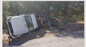
Mines should ensure that vehicles and trailers are fit-for-purpose when being used to transport a load. The suitability of the towing vehicle to handle the trailer mass and the trailer load should be assessed.
