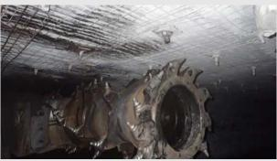
Mine operators must assess the risk for tasks and consider the clearance required to operate equipment. The risk assessment must also consider where workers are located during the cutting cycle.
