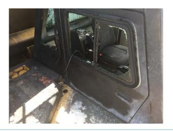
Dangerous incident SinNot-2018/01992 A collision occurred between a front-end loader and a haul truck on the run of mine pad at an underground coal mine. The loader was working on the pad when the haul truck entered without communicating with the loader operator.
