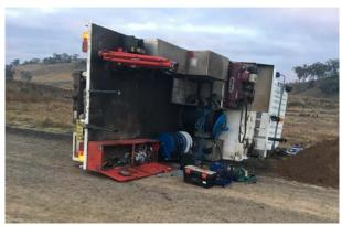
When tanks are fitted to vehicles (such as fuel or water tanks), the risk of fluid movement should be considered and appropriate controls put in place including baffles and minimum/ maximum fill levels.
