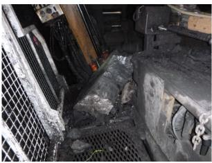
Rib protection fitted to continuous miners must be designed and operated to match the rib conditions at the mine and forms part of the entire temporary support requirements while installing support.
