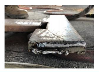
Dangerous incident SinNot-2018/01409 A high voltage cable was damaged when it was hit by a longwall roof support being transported to the surface of the mine. The electrical power was not interrupted.
